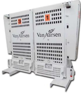
The screens are stored in a cassette system that is suspended above the hammer mill. This construction provides:
