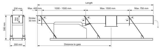
NOTE: Orders shall contain the length of the trough and the position of any gates.
