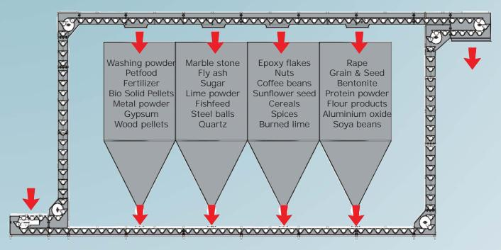
Construction form "D" Elevator type 110E Capacity 26 m³/h at 20 m/min. Power consumption: 1.5 kW
