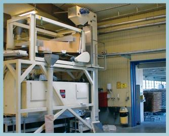
Elevator construction form C for processing of seed.
