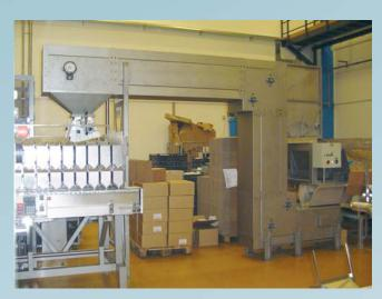
Simatek bucket elevator construction form A mounted in connection with a weighing system for chocolate and liquorice.
