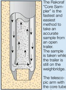
The Rakoraf "Core Sampler" is the fastest and easiest method to take an accurate sample from an open trailer. The sample is taken while the trailer is still on the
