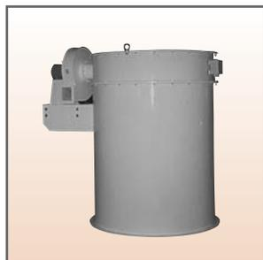
Filter Series SFM, extraction of bags from above, modular fixing with flange, filtration surface area varying from 32 m<sup>2</sup> to 57 m<sup>2</sup>, with pulse air jet cleaning.
