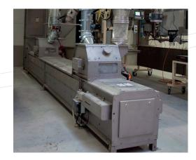
**Processing industry** Simatek Universal Elevator with 2 drum feeders (CBFS) conveying pre-mix
