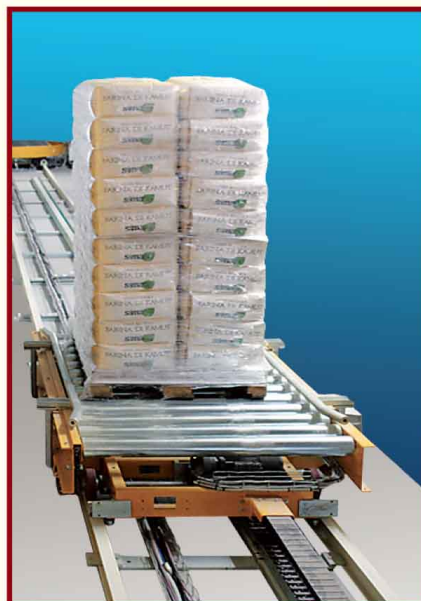
Navetta per pallet pieni Shuttle for full pallets
