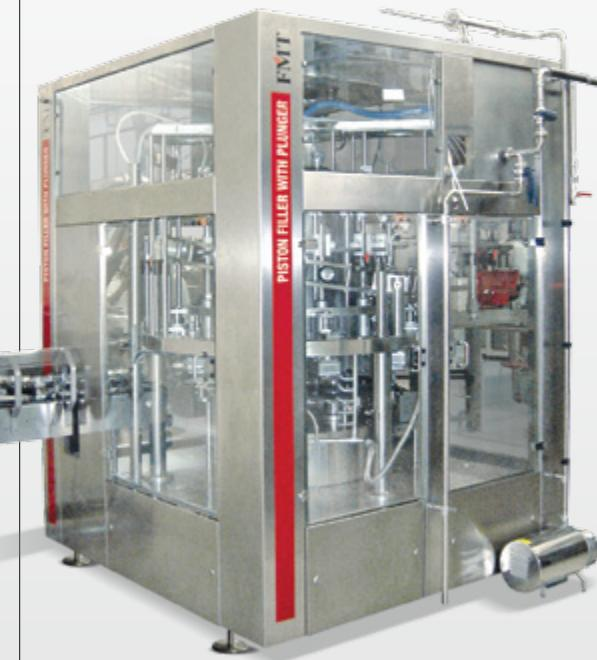
Machine suitable for products having medium and big pieces inside. The special system with plunger permits the total discharge of the nozzles after the filling phase with no residual dripping. High precision in the dosing phase is always granted.
