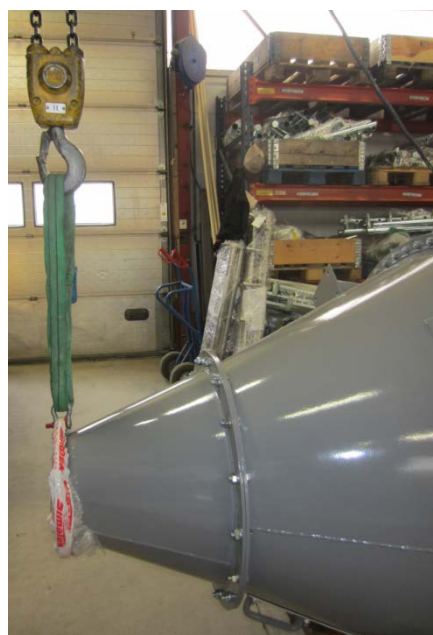
Fig. 2: Example of lifting eye at base of filter.
