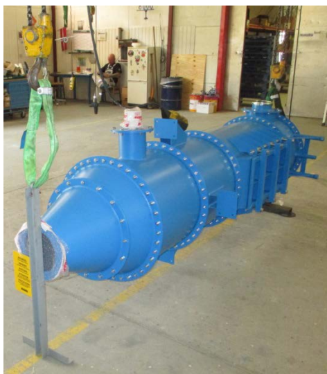
Fig. 3: Example of support attached to bottom of filter (used here as lifting eye).
