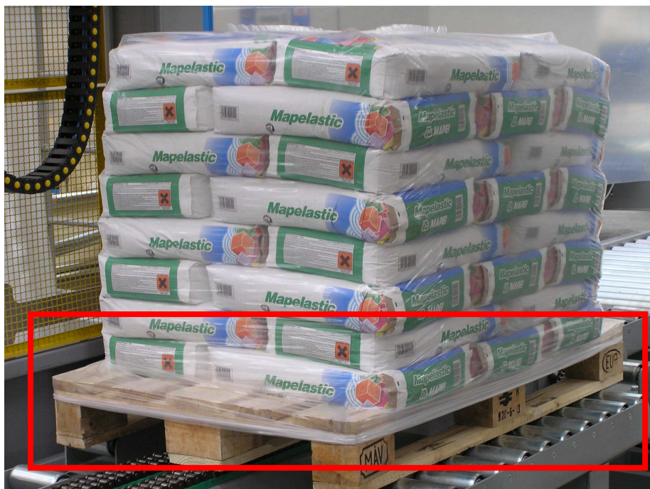
Ref.: Stretch hood rope around the wooden pallet – even with smaller load than the pallet
